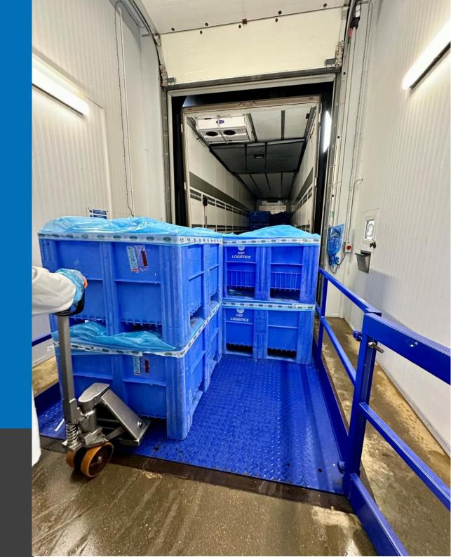
This lift has a raised height of 1400mm and a lifting capacity of 2000Kg. The platform size is 2350mm deep x 1500mm wide. It is equipped with side barriers, interlocked gates, a tread plate platform surface and chainmail mesh skirts. It is controlled from the upper level and platform. The complete lift is hot dipped galvanised.
