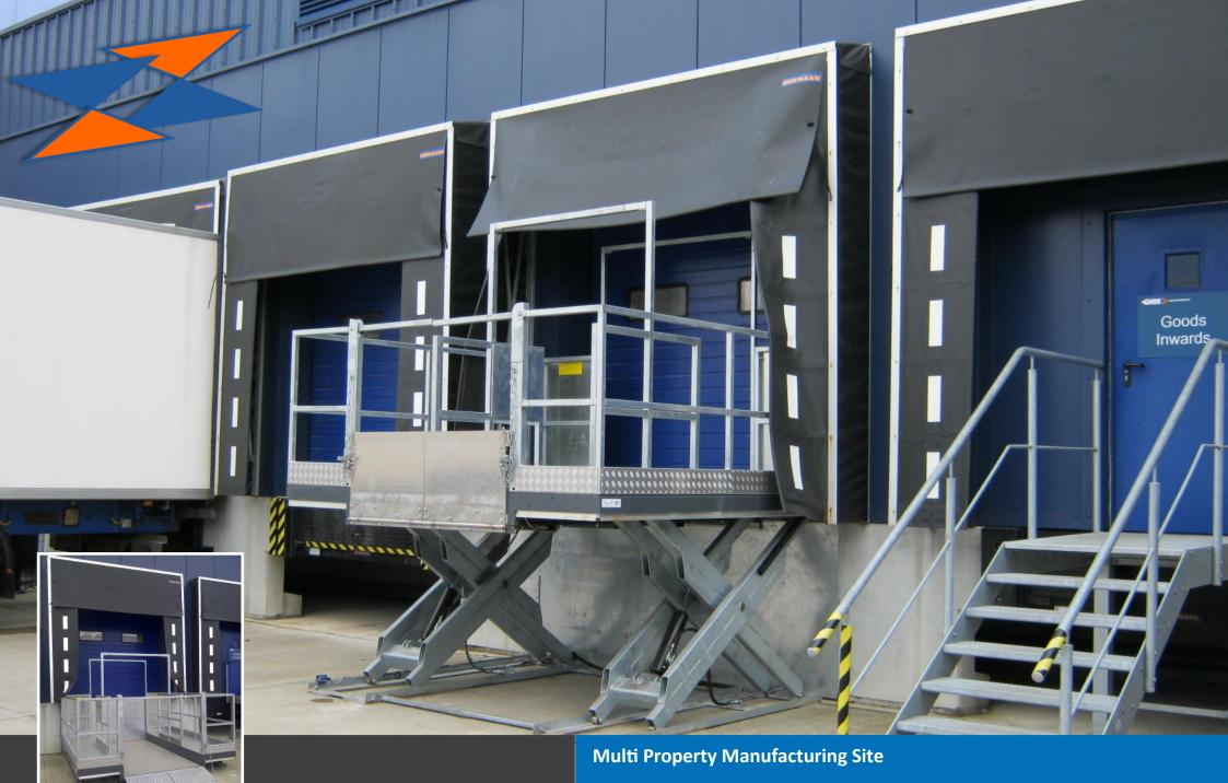
This client builds components for AirBus which need to be moved between buildings. This Edmolift Multi-Dock transports the parts between yard level and factory level. No need for a pit.
