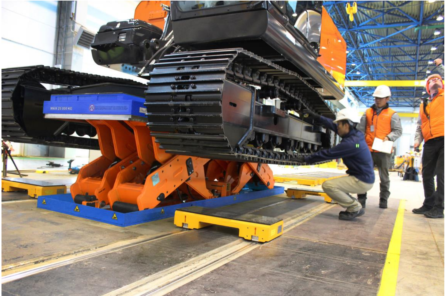
25,000Kg capacity scissor lift platform for Hitachi Construction Machinery Europe
